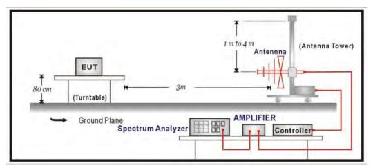
Above 1GHz Test Setup:
