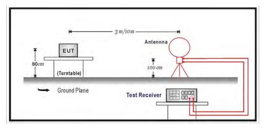
Under 1GHz Test Setup:
