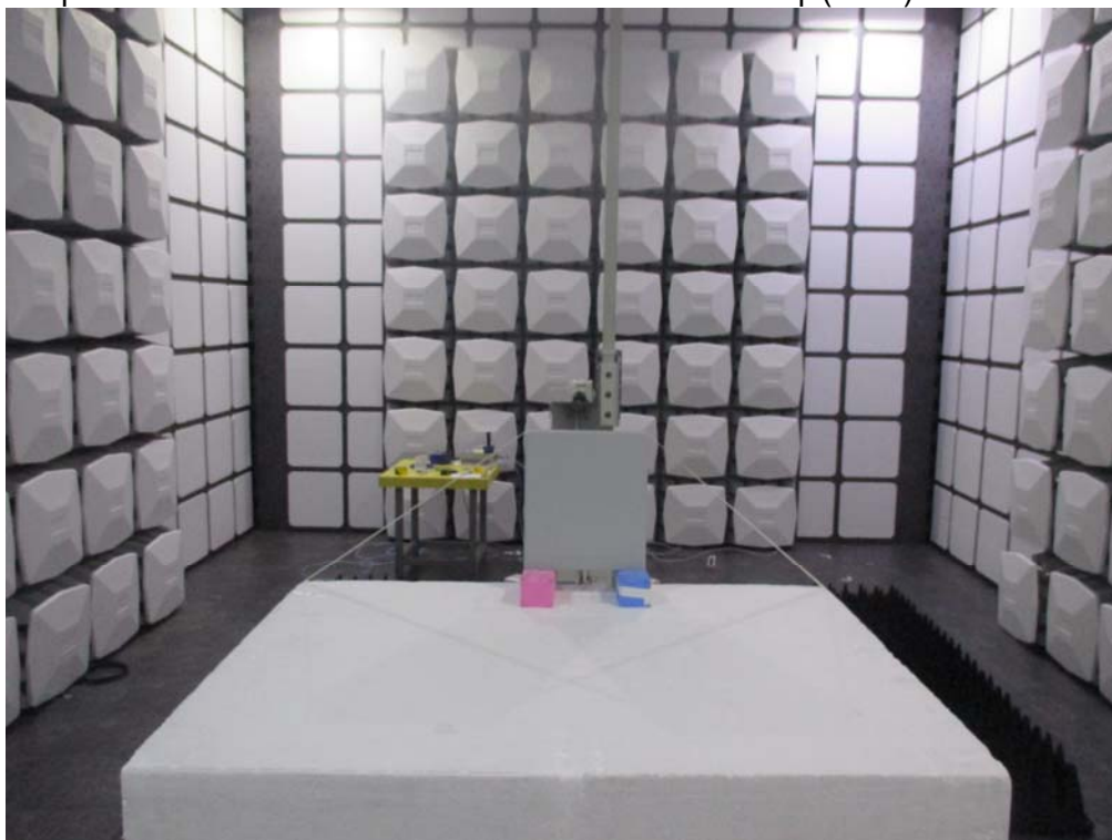
Description: Front View of Radiated Emission Test Setup (Horn)
