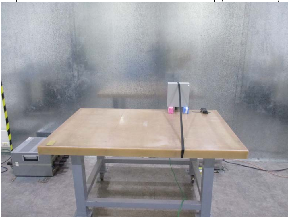
Description: Back View of Conducted Emission Test Setup (ADP-65JH HB)
