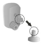
2. Remove the grommet and the cap on the rear side of the camera.
