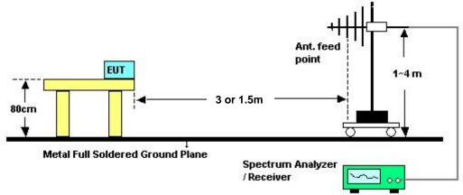
Above 5GHz shall be extrapolated to the specified distance using an extrapolation factor of 20 dB/decade form 3m to 1.5m.
