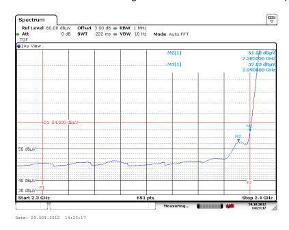
Plot 10b: zoomed in to the restricted band 2310 - 2390 MHz, delta value is obtained by difference between M1 from plot 10a and M1 from plot 10b (104.69 - 52.63 = 52.1 dB).
