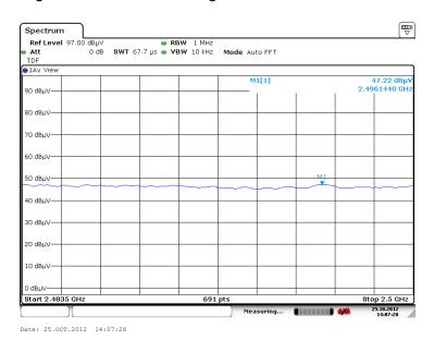
Plot 4b: zoomed in to the restricted band 2310-2390 MHz, delta value is obtained by difference between M1 from plot 4a and M1 from plot 4b (99.32 - 47.22=52.1 dB).
