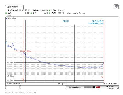
Plot 8b: zoomed in to the restricted band 2483.5 - 2500 MHz, delta value is obtained by difference between M1 from plot 8a and M1 from plot 8b (106.66 - 53.8 = 52.9 dB).
