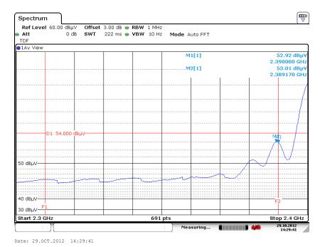
Plot 14b: zoomed in to the restricted band 2310 - 2390 MHz, delta value is obtained by difference between M1 from plot 10a and M1 from plot 10b (101.67 - 52.92 = 48.8 dB).
