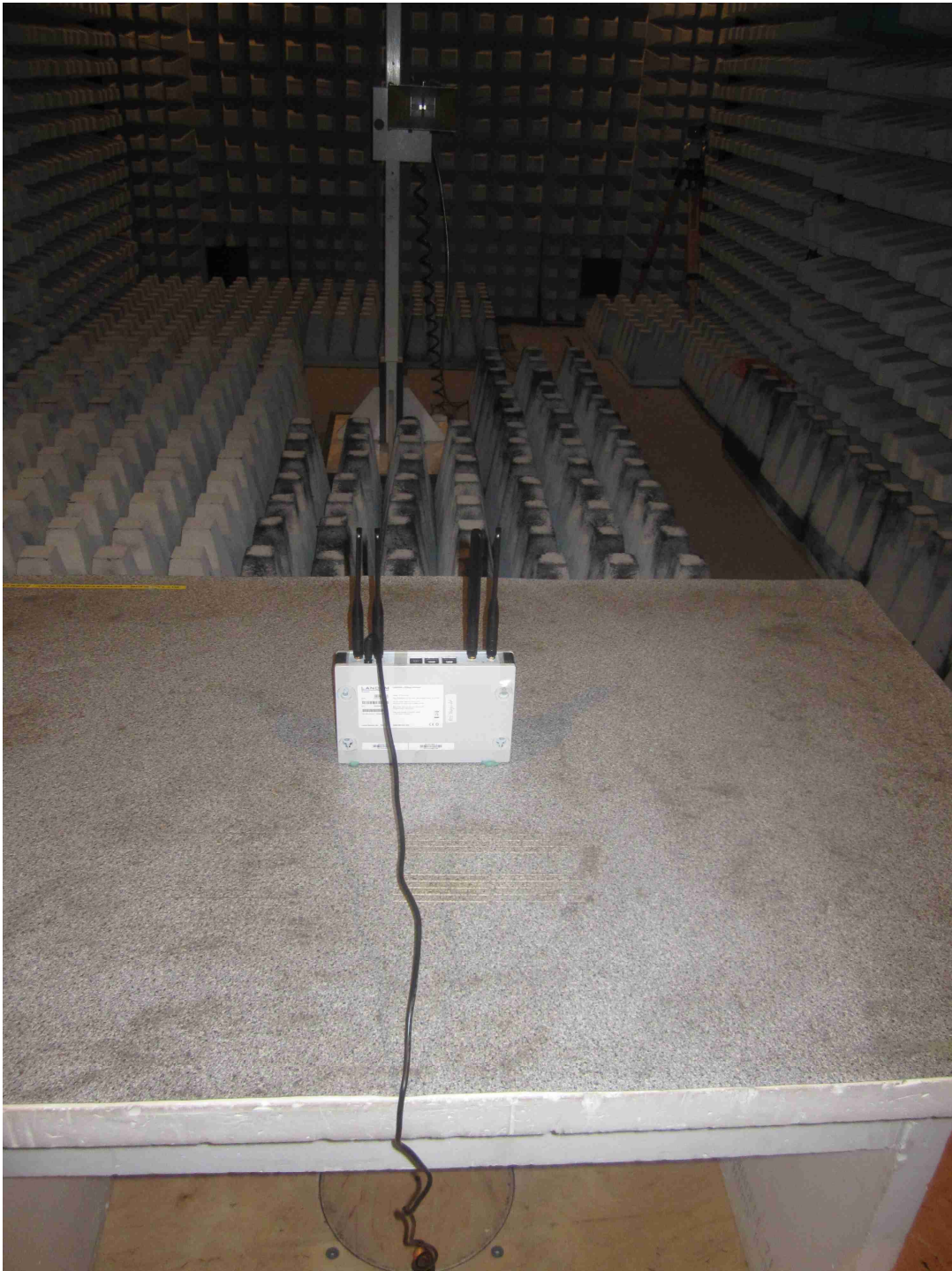
120195_05: Test setup - Radiated emission (fully anechoic chamber)
