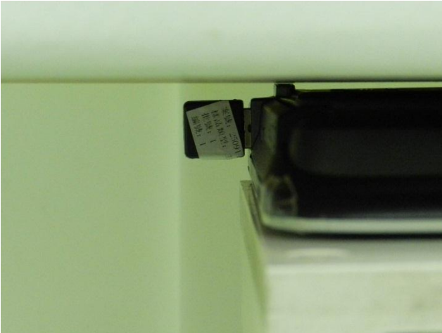
Direct Laptop Plug-in for USB Configuration 3 (Vertical Front with Phantom 5 mm Gap)
