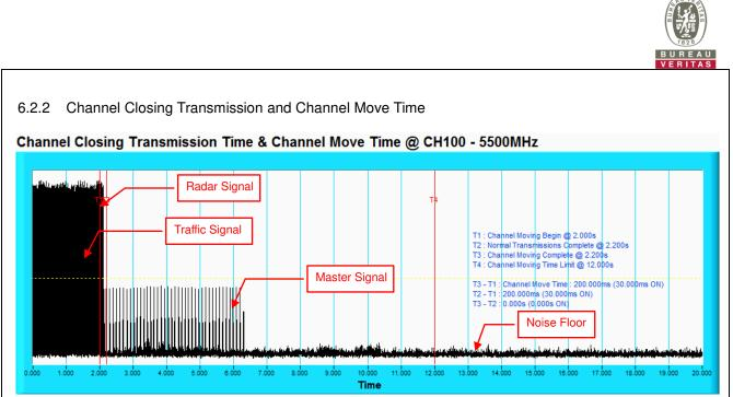
NOTE: T1 denotes the start of Channel Move Time upon the end of the last Radar burst. T2 denotes the data transmission time of 200ms from T1. T4 denotes the 10 second from T1 to observe the aggregate duration of transmissions.
