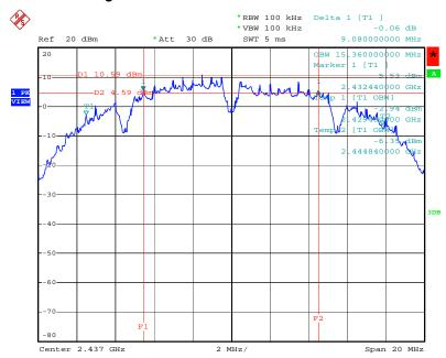
6 dB Bandwidth Plot on Configuration IEEE 802.11b Ant. A + Ant. B+ Ant. C / 2437 MHz
