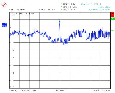
Power Density Plot on Configuration IEEE 802.11g Ant. A + Ant. B+ Ant. C / 2437 MHz
