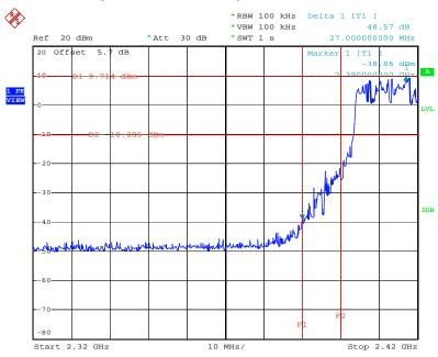
Low Band Edge Plot on Configuration IEEE 802.11g Ant. A + Ant. B+ Ant. C / 2412 MHz
