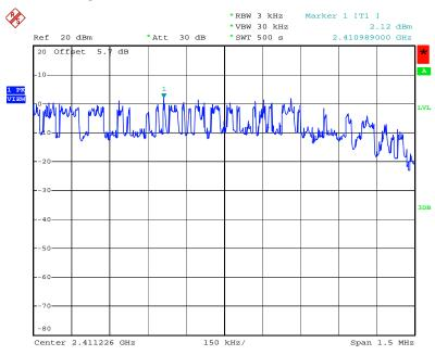
Power Density Plot on Configuration IEEE 802.11b Ant. A + Ant. B+ Ant. C / 2412 MHz
