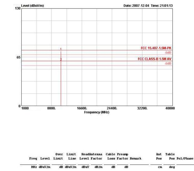
Note: Item 1 fall in restricted band, thus 15.209 limit applies. However, the test site distance has been moved to 1.5m, the corresponding limit will be adjusted to 80dBuV/m.
