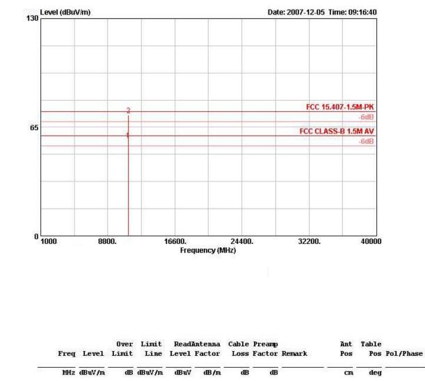
Note: Item 2 fall in restricted band, thus 15.209 limit applies. However, the test site distance has been moved to 1.5m, the corresponding limit will be adjusted to 80dBuV/m.
