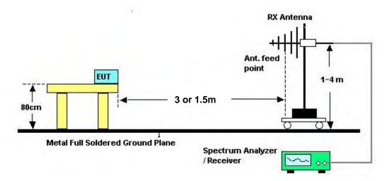
Above 5GHz shall be extrapolated to the specified distance using an extrapolation factor of 20 dB/decade form 3m to 1.5m.
