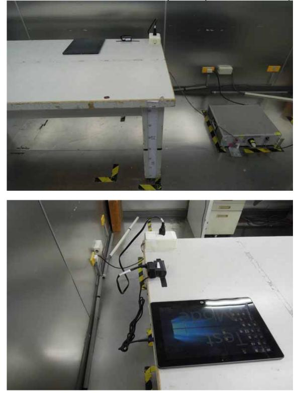
AC Power Line Conducted Emission Setup Photos (Model No.: TPN-LA06)
