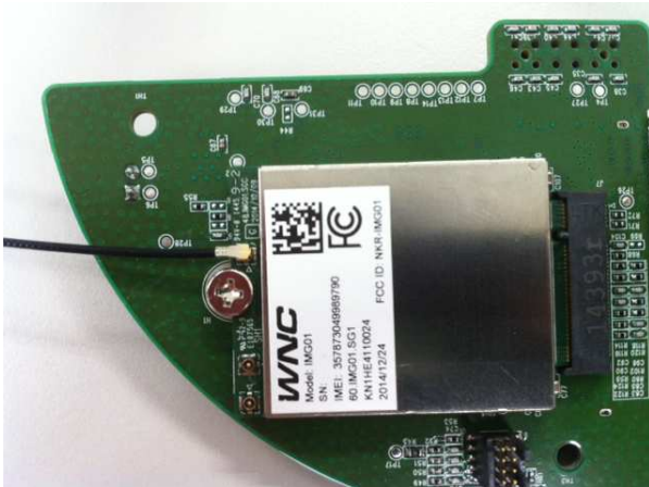
Connect to LTE primary antenna
