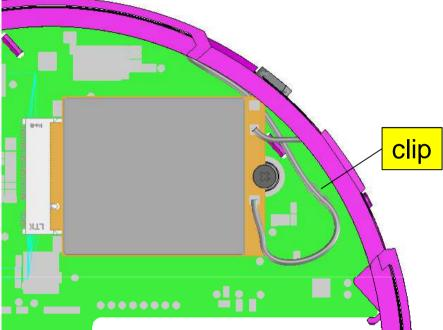
Connect antenna cable to PCB. Cables are fixed with IPEX on the module.
