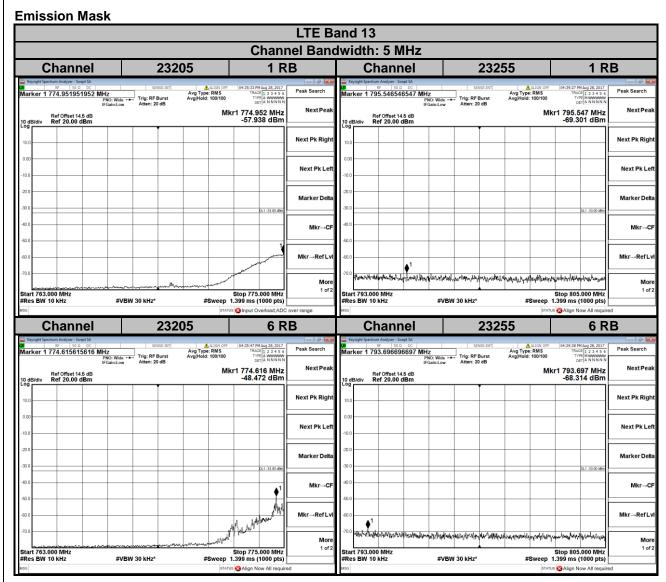
For the 763 - 775 MHz and 793 - 805 MHz band ,the FCC limit is 65+10log(P[watt]) in a 6.25 kHz bandwidth . Since it was not possible to set the resolution bandwidth to 6.25 kHz with the available equipment , a bandwidth of 10 kHz was used instead to show compliance. By using a 10 kHz bandwidth on the spectrum analyzer.
