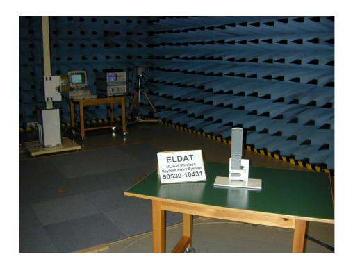
Test setup for radiated emission final test 30 MHz - 1 GHz (open area test site)
