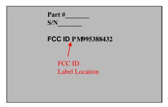
FCC ID label shall be placed on ulf g panel of chassis adjacent to the product part and serial number label. The FCC ID label is approximately 1.4 x 0.3 inches and the FCC ID is printed in 10pt Arial font.
