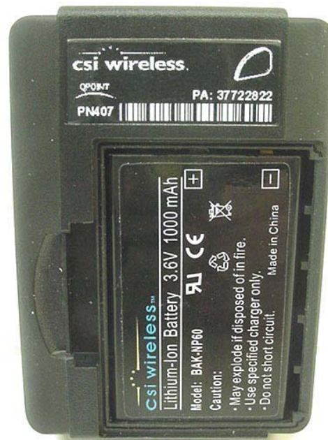
Lithium-ion Battery (Model: BAK-NP60)
