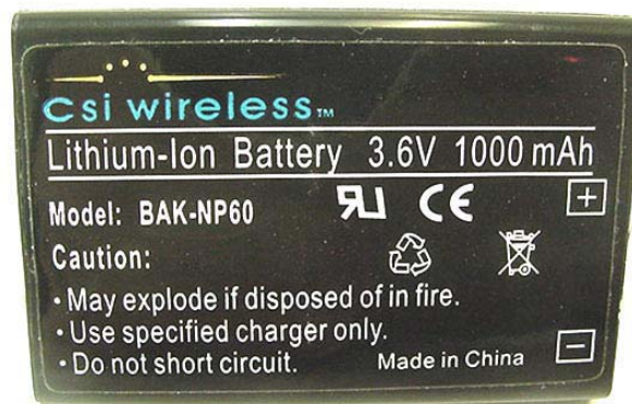
Lithium-ion Battery (Model: BAK-NP60)
