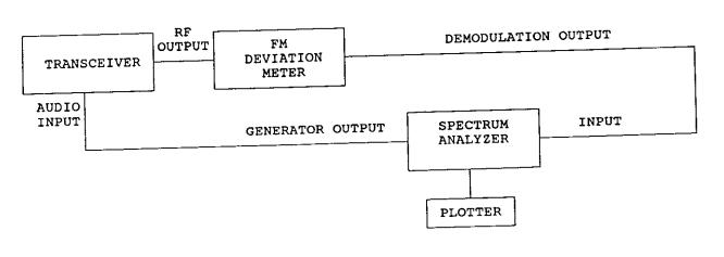
On that block diagram, the HP 3885A spectrum analyzer having the tracing generator, and the Marconi 2955A Radio Communication Test Set having an output of a demodulator, are used. After the calibration was made (the -20 dBm reading of the spectrum analyzer corresponds to the 9 kHz deviation) the spectrum analyzer was set to scan the frequency from 300 Hz to 30 kHz, with the same audio input level as described above.
