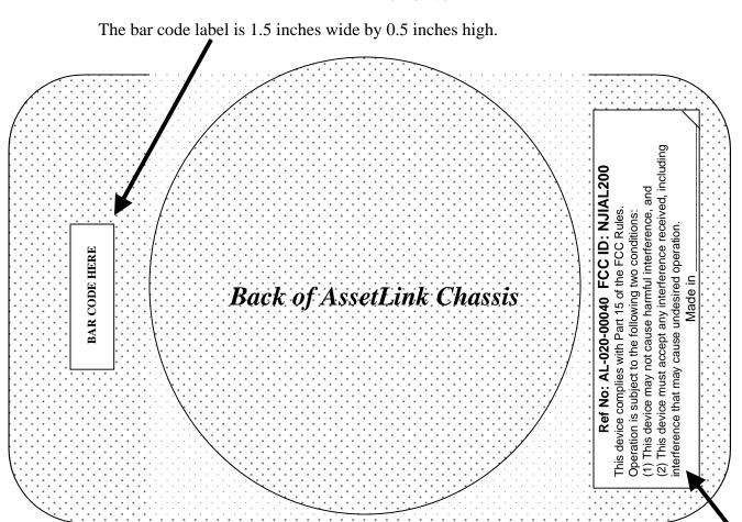
On the Model Number: typeface shall be 9 point Arial Bold, lettering shall be black on a white or silver background. On the FCC NO are:: typeface shall be at least 10 point Arial Bold, lettering shall be black on a white or silver background. On the warning area: typeface shall be 7 or 8 point Arial Normal on a white or silver background. The FCC label is 3.0 inches wide by 1.0 inches high.
