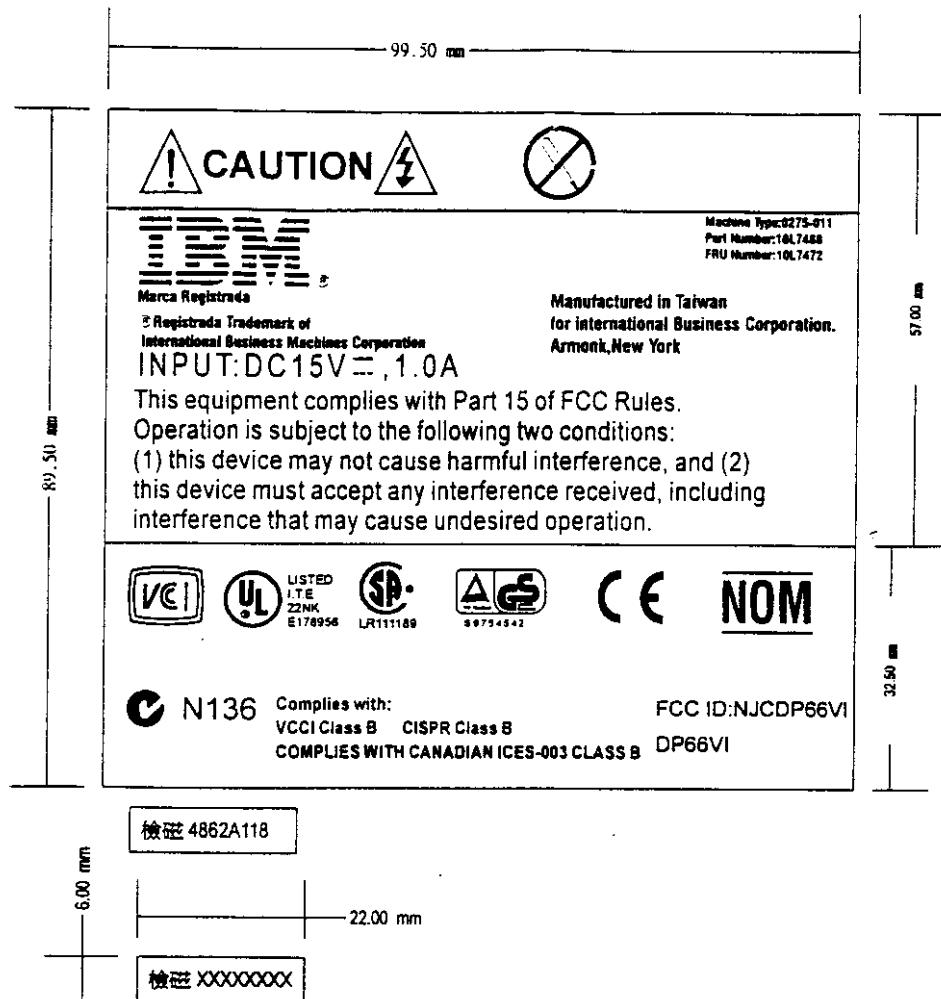
※ The FCC ID Label will be placed on the bottom of the EUT as shown in the following page :
