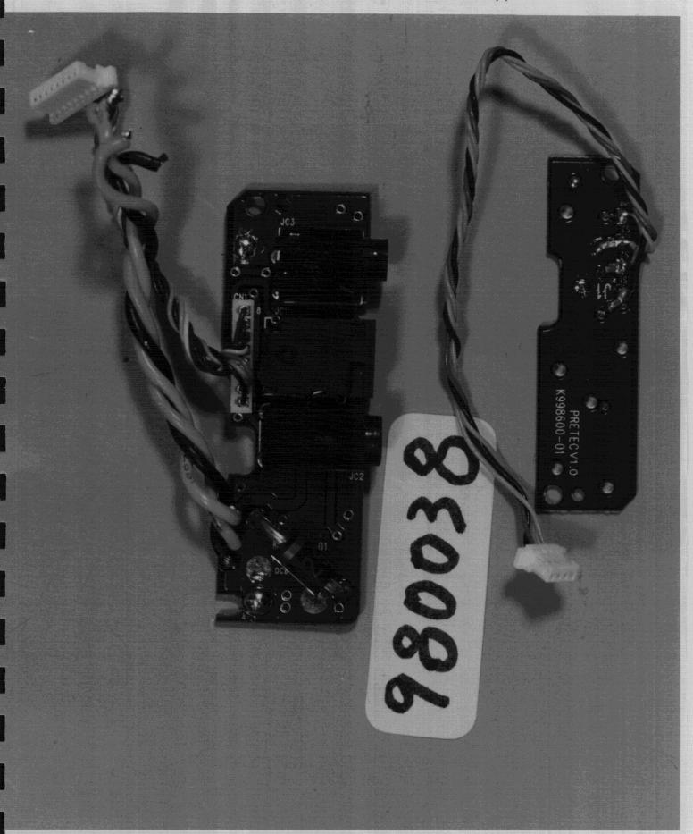
The Back View of Connector Board and Switch Board (2) 80008 Page 54 of 59 Accredited Lab. of NEMKO, A2LA, BCIQ
