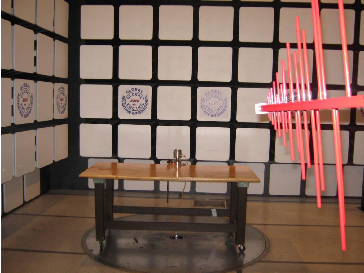
Radiated Emission Setup – Photo 1
