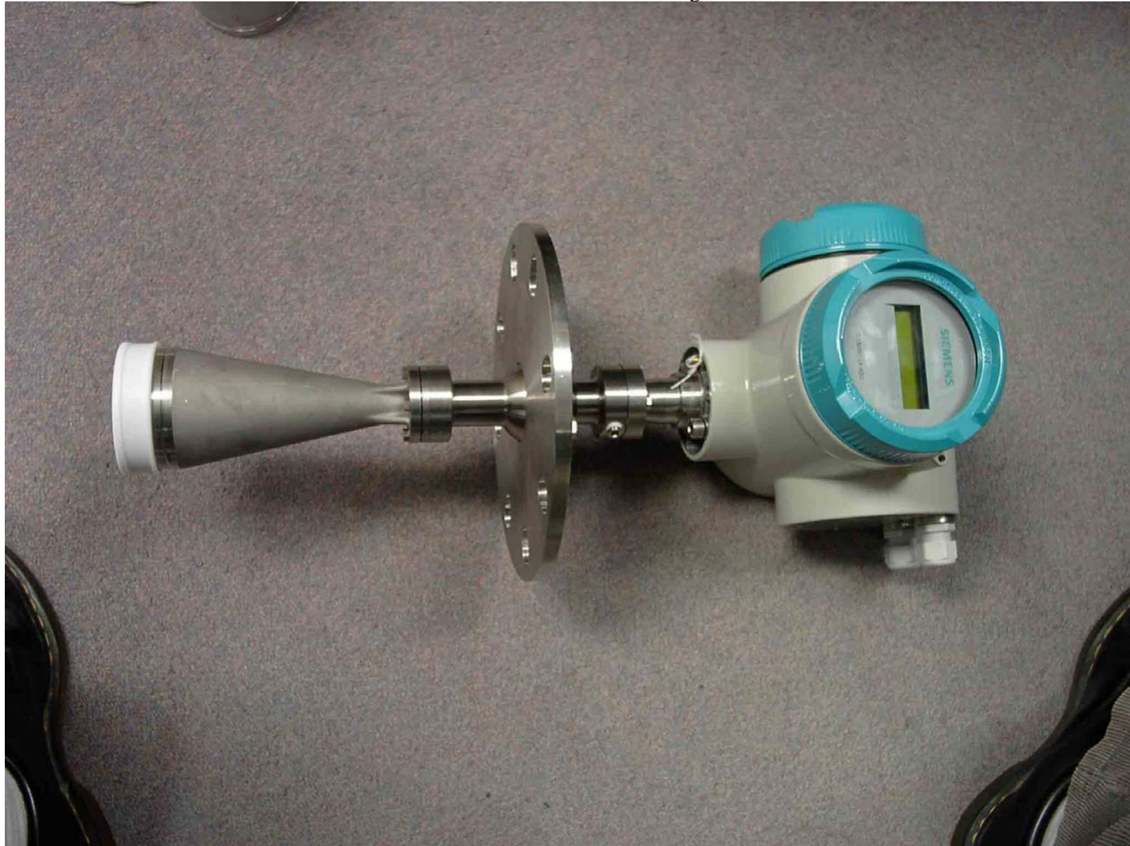
SITRANS LR 460, Model No.: 7ML5426 with 3" Flange Antenna and Dust Cover
