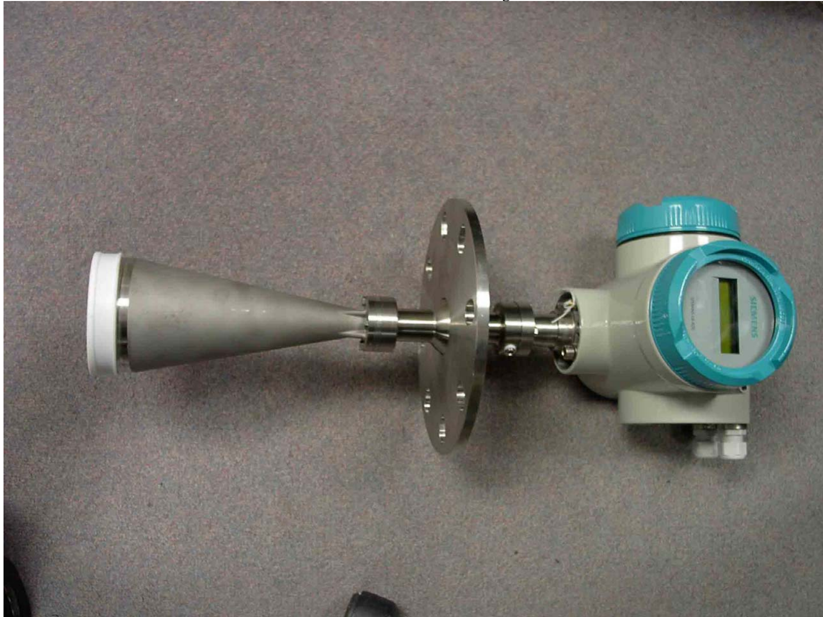
SITRANS LR 460, Model No.: 7ML5426 with 4" Flange Antenna and Dust Cover
