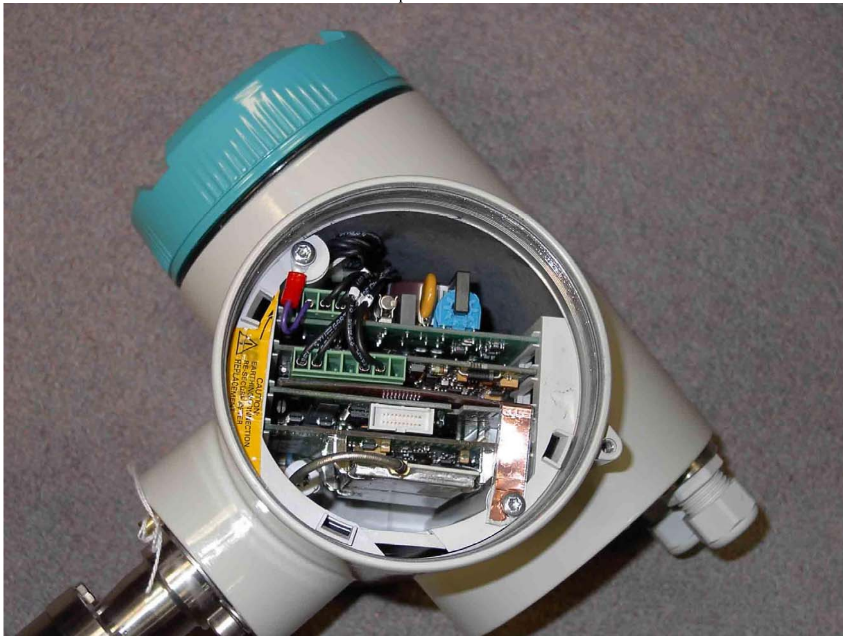
Board Stack placed into enclosure
