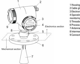
2 Cable gland 3 Electronics cover 4 Operating and monitoring module 5 Threaded ring 6 Process Flange 7 Antenna 8 Intermediate flange 9 Connection cover
