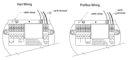
• DC input terminals shall be supplied from an SELV source in accordance with IEC 1010-1 Annex H.
