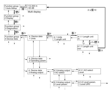
Follow the path traced with a bold line in the diagram above for input. The other paths lead to other device functions and parameters which are not required in this example. Next to the operating path, the control elements which you need to press are indicated and the operating steps are numbered.
