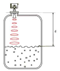
The propagation speed of microwaves in gases corresponds to the speed of light. The distance d is therefore proportional to the propagation time t:
