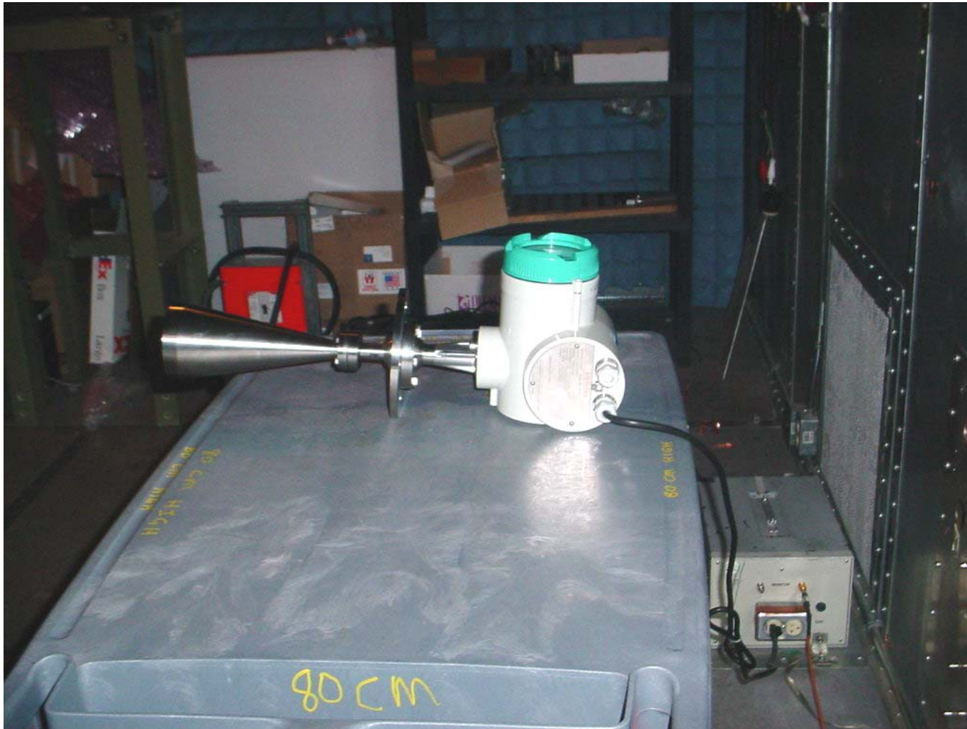
AC/DC Power Line Conducted Emissions Test Setup
