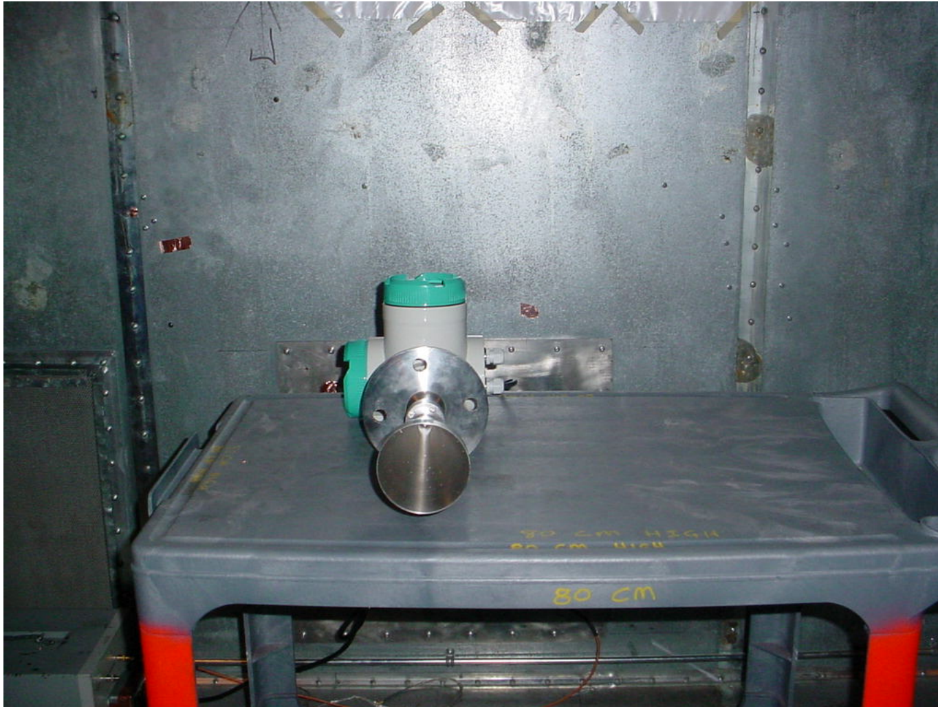
AC/DC Power Line Conducted Emissions Test Setup
