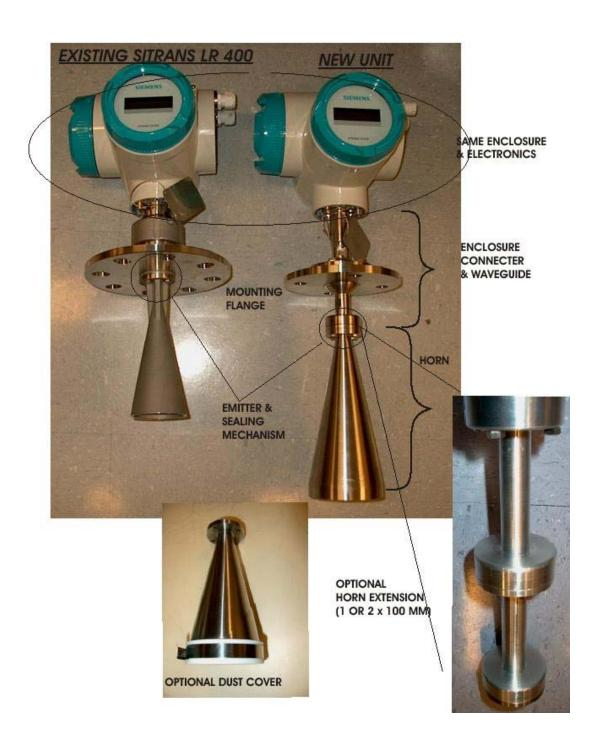
Figure 1: DRAWING SHOWING THE DIFFERENCE BETWEEN THE EXISTING AND NEW **VERSIONS OF SITRANS LR400**
