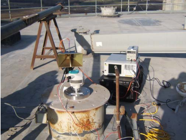
Test setup for 1-18GHz scan.
