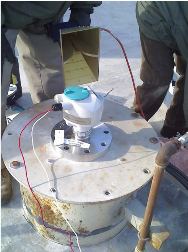
Test setup for 1-18GHz scan.
