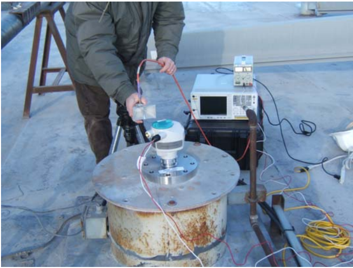
Test setup for 18-44.5GHz scan.
