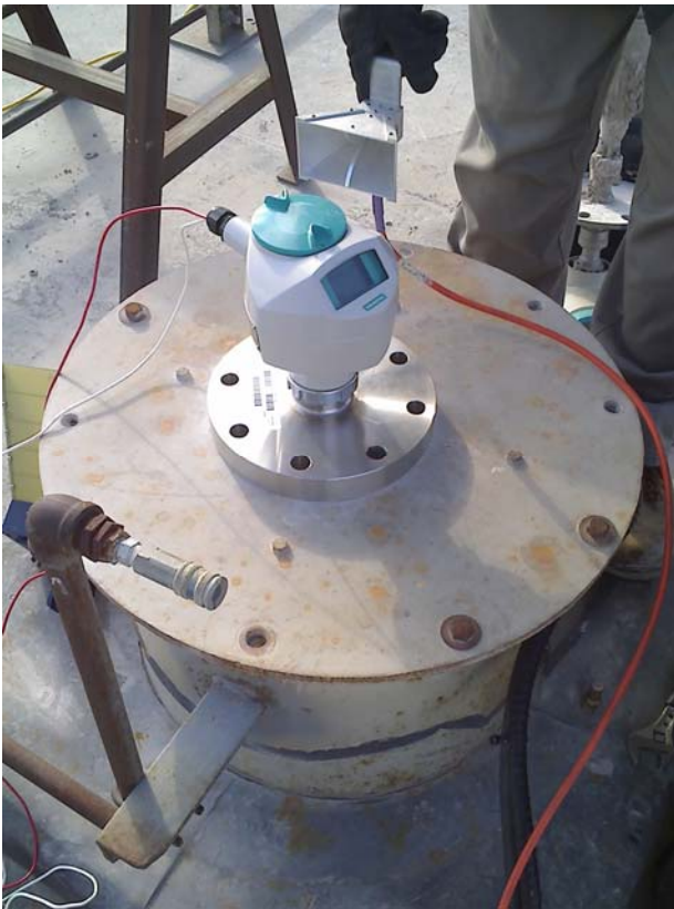
Test setup for 18-44.5GHz scan.
