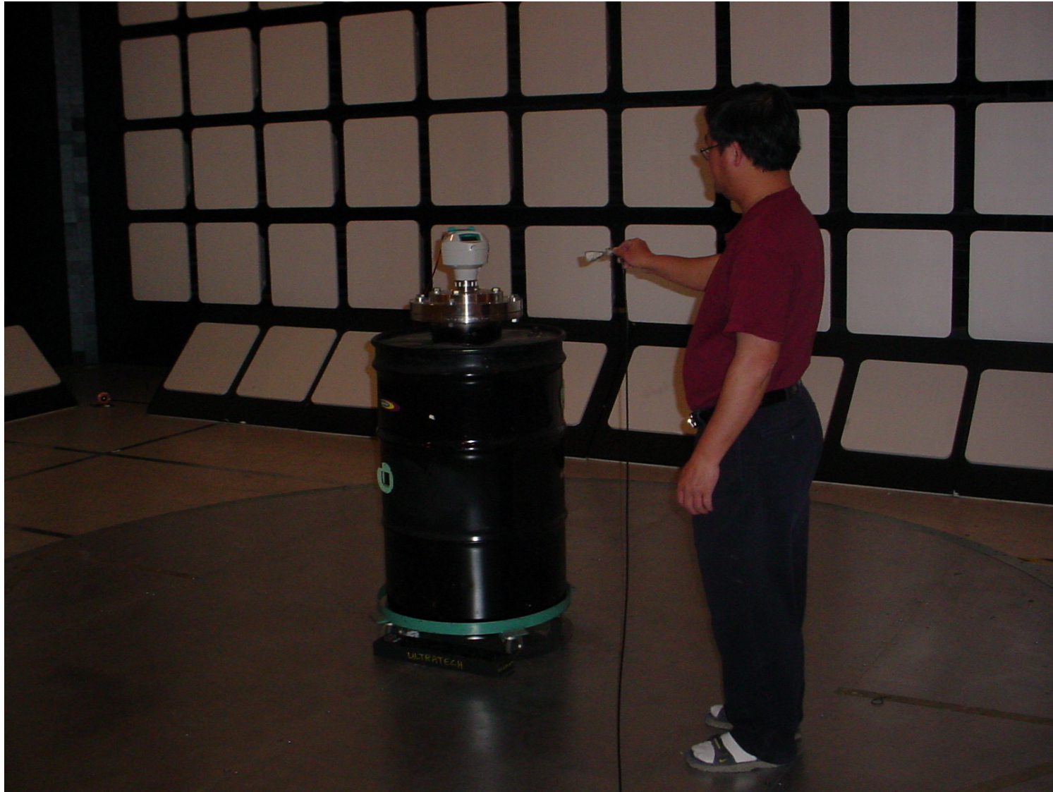
Plot #5: Radiated Emissions from SITRANS LR 250 mounted on top of the metal tank
