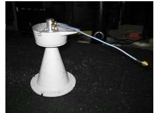
A transition is attached to each antenna.
