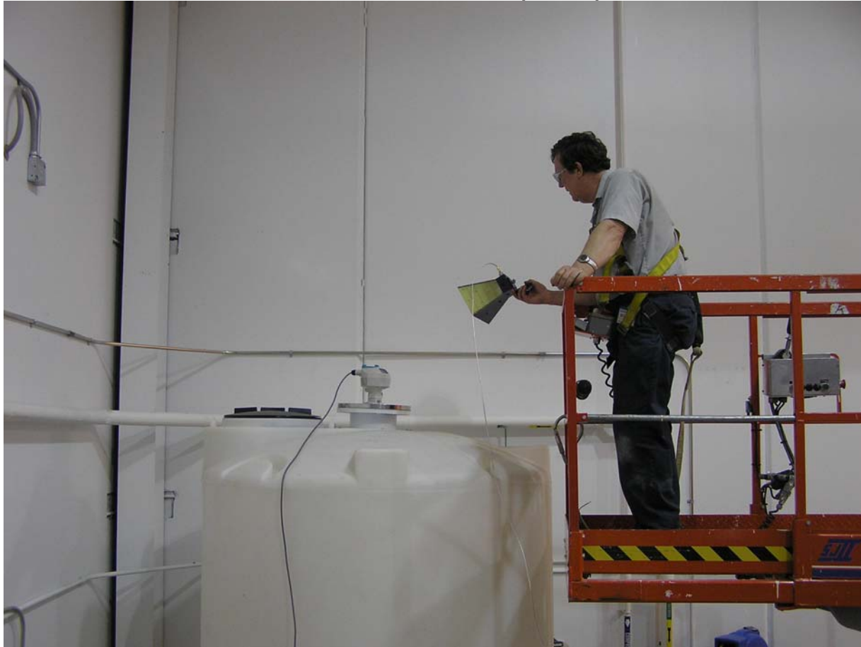
Radiated Emissions from SITRANS LR 200 mounted on top of the plastic tank
