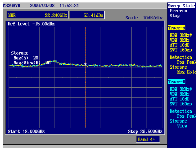
Scan between 18GHz -26.5GHz ((yellow - signal, blue – noise floor))
