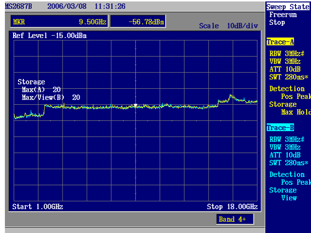
Scan between 1-18GHz (yellow - signal, blue – noise floor)
