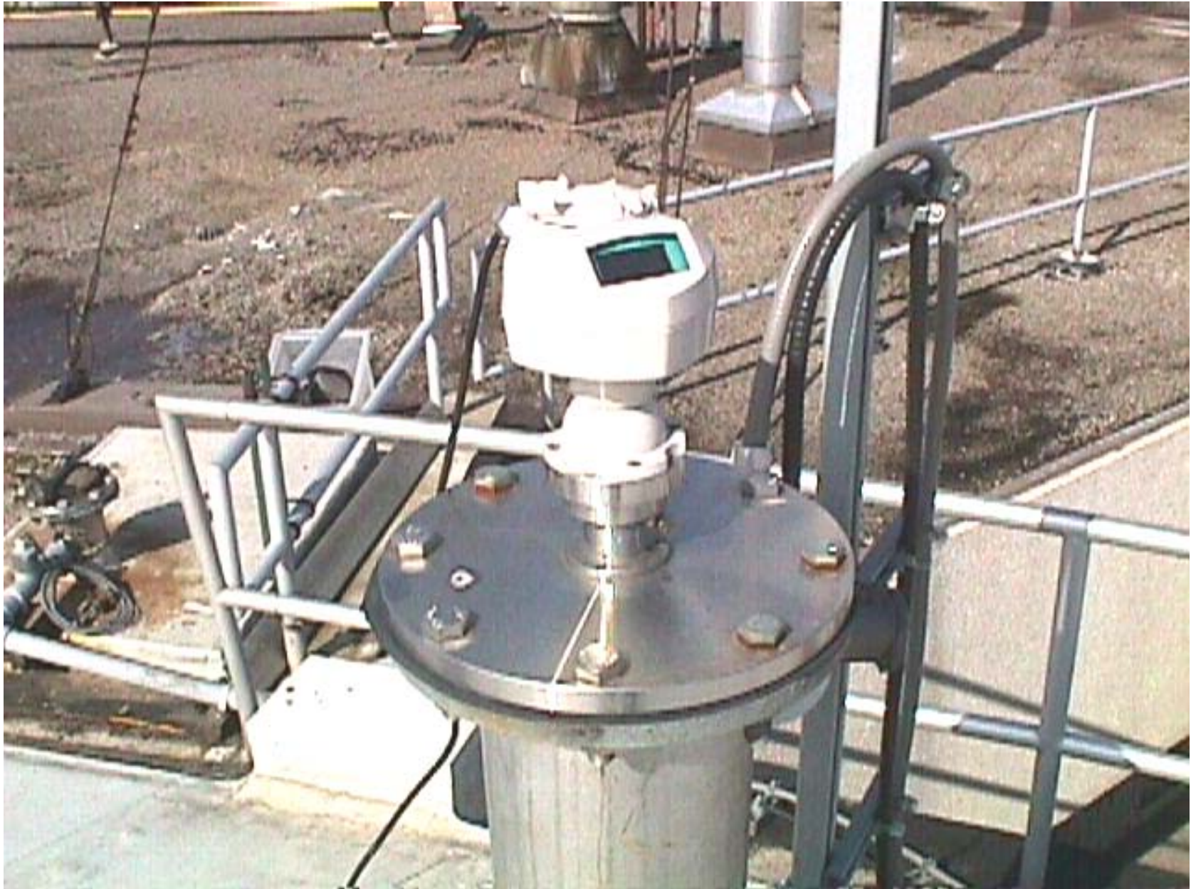
ANNEX 1 - PHOTOGRAPHS OF TEST SETUP with Concrete Tank SIEMENS MILLTRONICS RADAR LEVEL GAUGE (6.3 GHz)
