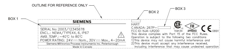
PRODUCT NAME BOX 1: SITRANS LR 200 or SITRANS Probe LR OPERATING FREQUENCY BOX 2: 5.8 GHz or 6.3 GHz (FCC STATEMENT APPEARS ONLY ON 6.3 GHz VERSION)
