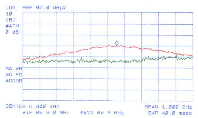
This plot shows the emission signal radiating toward the bottom of a tank/vessel, please note that this signal is not intended to radiate through air outside the tank/vessel.
