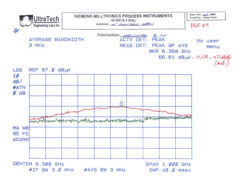
This plot shows the emission signal radiating toward the bottom of a tank/vessel, please note that this signal is not intended to radiate through air outside the tank/vessel.
