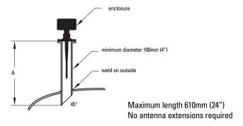
Standpipes that are 8" or larger in diameter provide excellent signal conditions. These conditions allow for standpipe lengths of up to 24" using the standard rod without any extensions.
