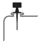
Ideally, the standpipe should be as short as possible. If your application requires a standpipe that exceeds our recommended maximum lengths, consider using a waveguide and horn combination. If you create a new standpipe for the radar unit, ensure the weld seams are on the outside of the standpipe, not the inside.
