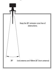
Due to the polarization effect of the microwave signal related to the wall of the vessel, we recommend locating the IQ 300 a minimum of 30cm (1') away from the sidewall for every 3m (10') of vessel height.
