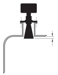
The end of the horn should protrude a minimum of 10mm (0.5") to avoid interference with the standpipe.
