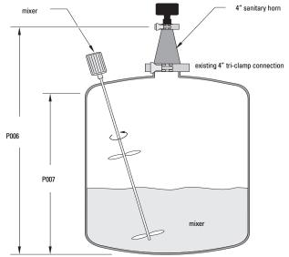
**Note**: Sanitary Antenna Options: The one-piece antenna/process seal provides excellent mounting method, even on nonsanitary installations.
