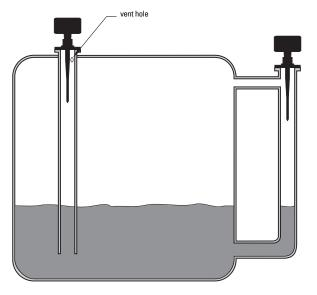
Suitable pipe diameters are 2" (50mm) to 10" (250mm).
