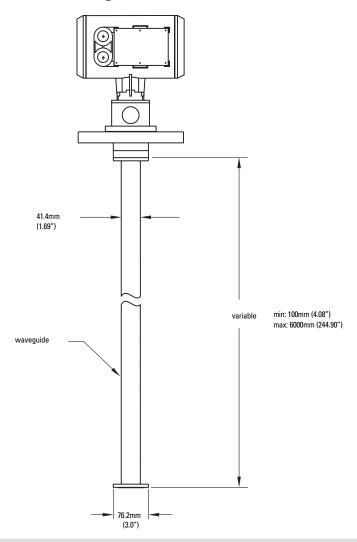
Note: you can connect a maximum of two waveguides together.
