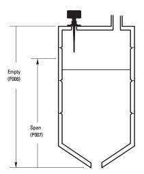
The application is to obtain a level measurement and corresponding 4-20 mA output proportional to asphalt levels in a storage tank. The bottom of the antenna flange is 5m from the tank bottom. The empty level is 0m (bottom) and the full level (span) is 4.5m from the bottom. The maximum rate of filling or emptying is about 0.1m/min. In the event of a loss of echo, the IQ Radar 300 is to go into fail-safe Hi after 2 minutes.
