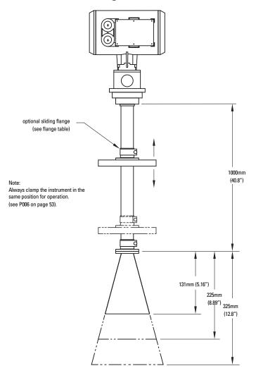
**Note:** Maximum pressure 0.5 bar at 60° C (140° F) for sliding flange option.
