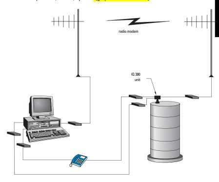
The standard IQ 300 supports Modbus communications on board and Hear and Profibus PA via add-on cards.
