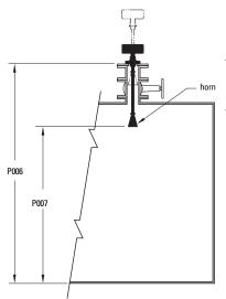
Maximum level should be maintained at least .46m (18") from the end of the horn.
