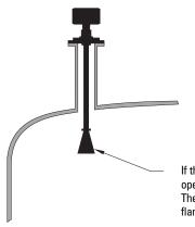
In applications where the standpipe is too long and the diameter is too small (such as a standpipe that is 100mm (4") in diameter and 460mm (18") in length), the rod antenna is not suitable due to standpipe interference. In this case, use the waveguide/horn combination. Waveguide extensions are available in custom lengths.
