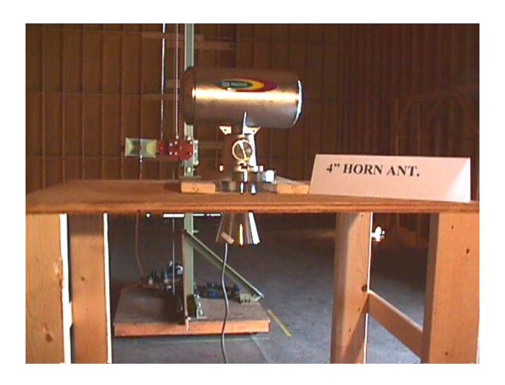
Test with 4" Sanitary Horn Antenna in its intended position
