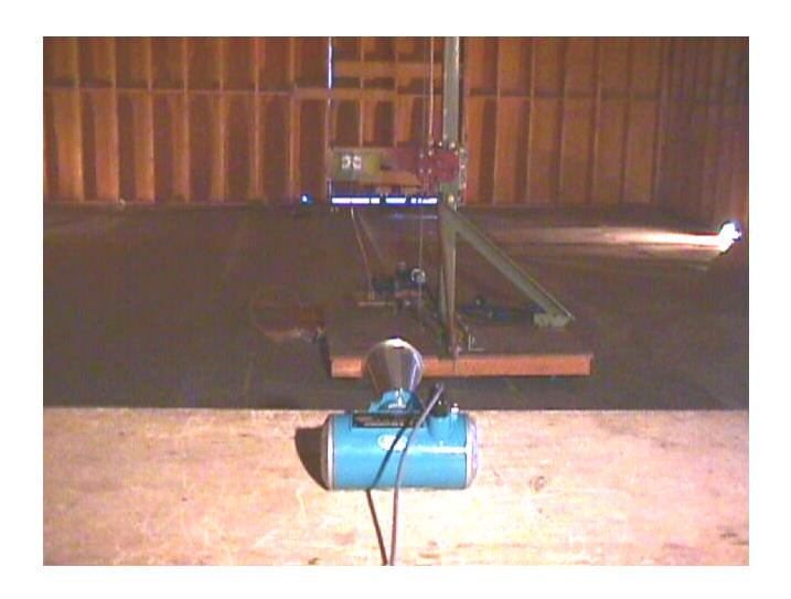
10.2.3 RF Fundamental and Spurious/Harmonic Emissions around the EUT at the distance 1 meter and 3 meters in the free space (this represents the worst case covering the actual installation on top of a tank/vessel)
