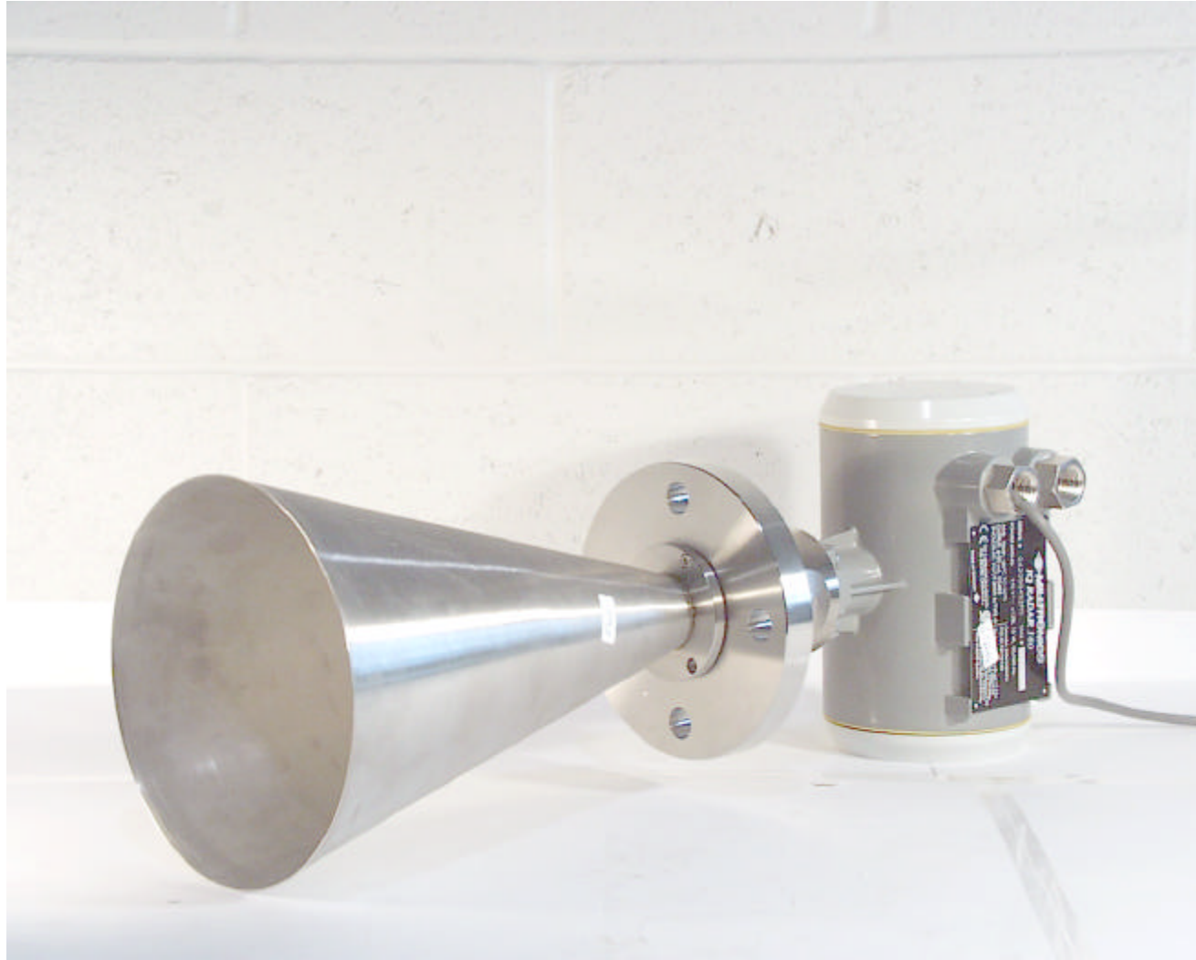
PICTURE #4: MILLTRONICS IQ RADAR160 WITH 8" HORN ANTENNA & ANTENNA EXTENSION
