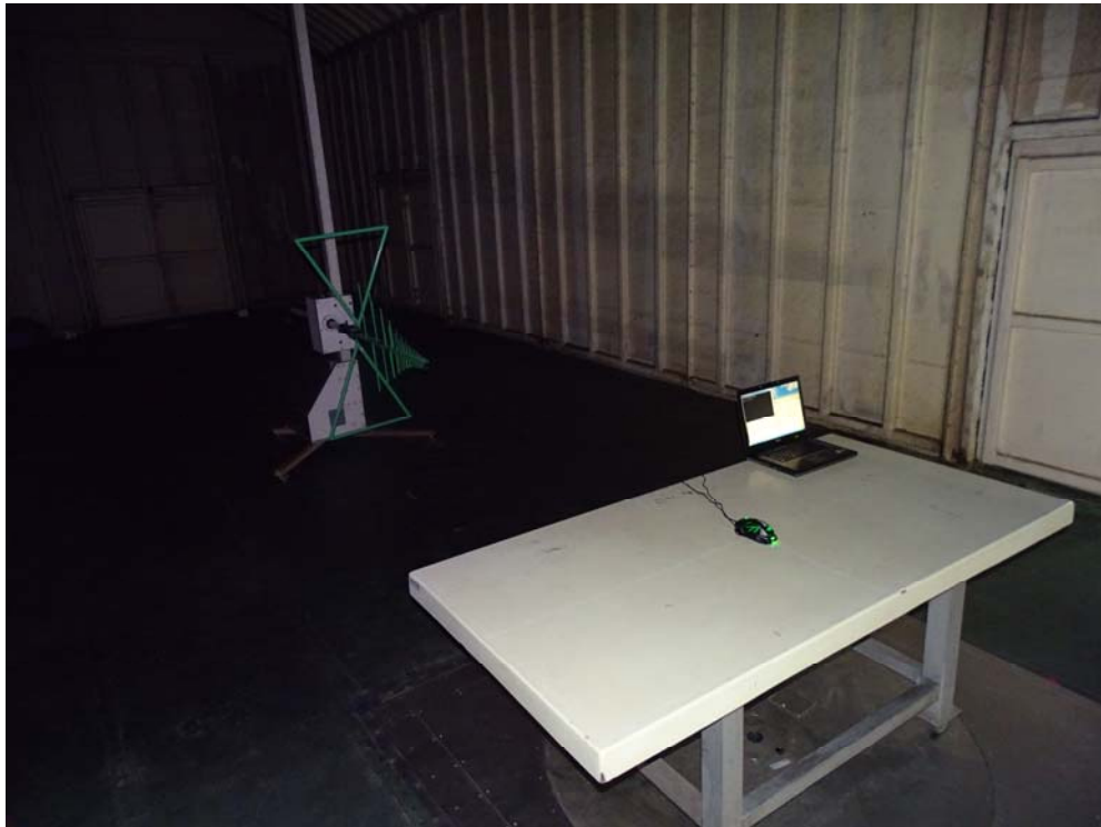
Back View of Radiated Test (Charge Mode)
