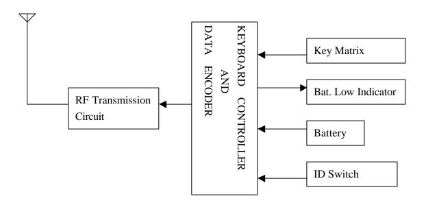
**Battery** provides the necessary power for operation. The proposed one is a single size AA battery.
