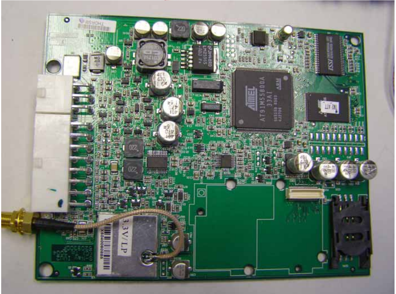
Photo 5. Board Top Module Removed (Note: the shielded component at the bottom of the board is the GPS module. No components are under the GPS module.)
