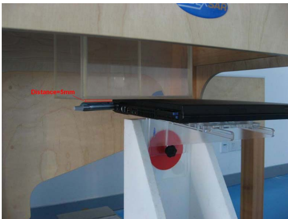
Fig.3 Side Position(connect to IBM T43, Distance=5mm)
