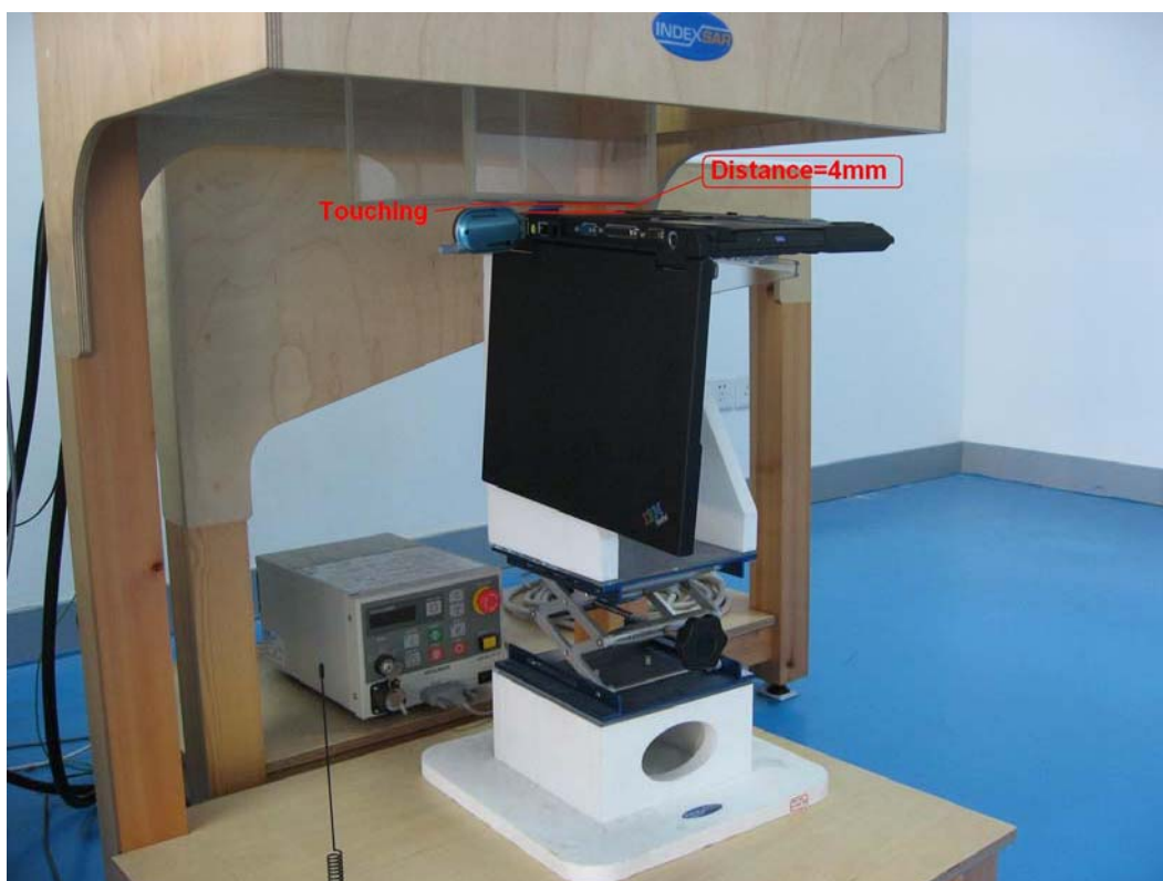
Fig.5 Side Position(connect to IBM T20, Touching Flat Phantom)
