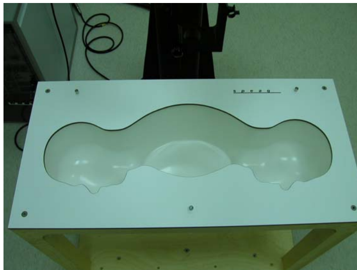
Fig. 5.3 Top view of twin phantom
