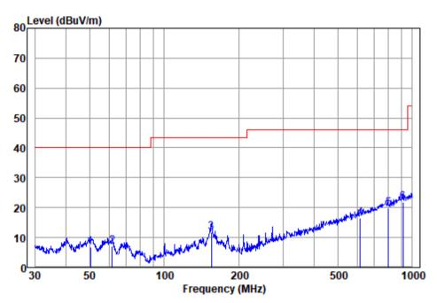
Antenna Polarity : HORIZONTAL EUT/Project :0949LM
