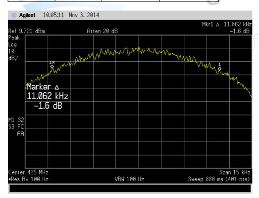
425.000 MHz F1D – 25.0 kHz spacing
