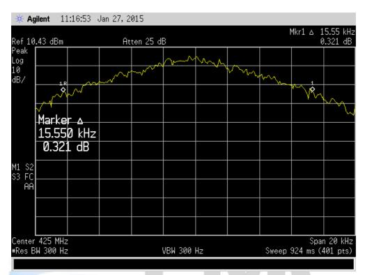
469.000 MHz F1D - 12.5 kHz spacing
