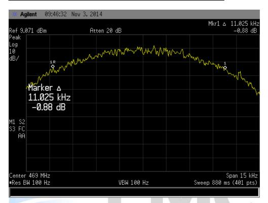
469.000 MHz F1D – 25.0 KHz spacing
