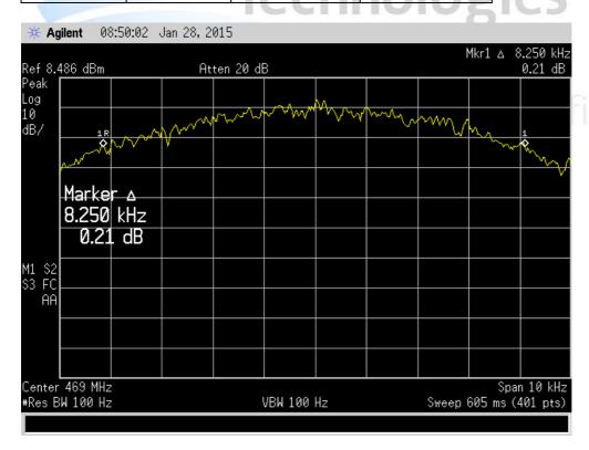
469.000 MHz F1D – 12.5 kHz spacing
