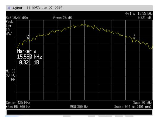
469.000 MHz F1D - 12.5 KHz spacing
