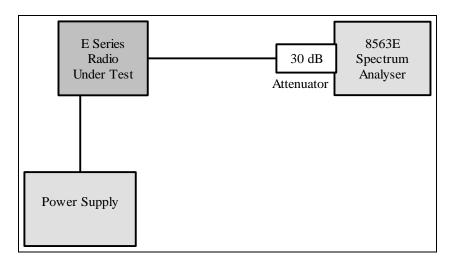
Test Data was generated using test firmware within the radio. Because the spectrum is data dependent for this modulation tests where performed for the three data patterns listed in section 2 of this report. Only 1200 bps was tested, 300 and 600 bps can be considered as a special case of 1200 bps (eg 1010 at 600 bps generates the same modulated waveform as 11001100 at 1200 bps).
