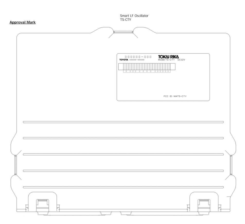
(Note) The layout and design of the approval mark may be changed. This device will be installed inside vehicle and end-user will not see the mark. FCC compliance statement will be included in User Manual as it is not practical to place on the device according to FCC Rules §15.19.
